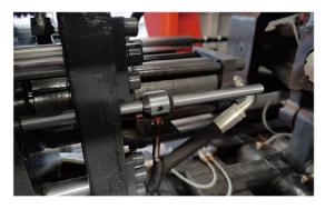
◆ 顶退限位: 采用撞杆结构,优化顶退位置调整,方便又美观。 Lifting and retracting limit: Adopting the ram structure, the adjustment of the position of the ejecting and retracting is optimized, which is convenient and beautiful.
