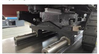
◆ 注射台旋转装置:更换螺杆料筒更加方便、高效。 Injection table rotation device: It is more convenient and efficient to replace the screw barrel.
